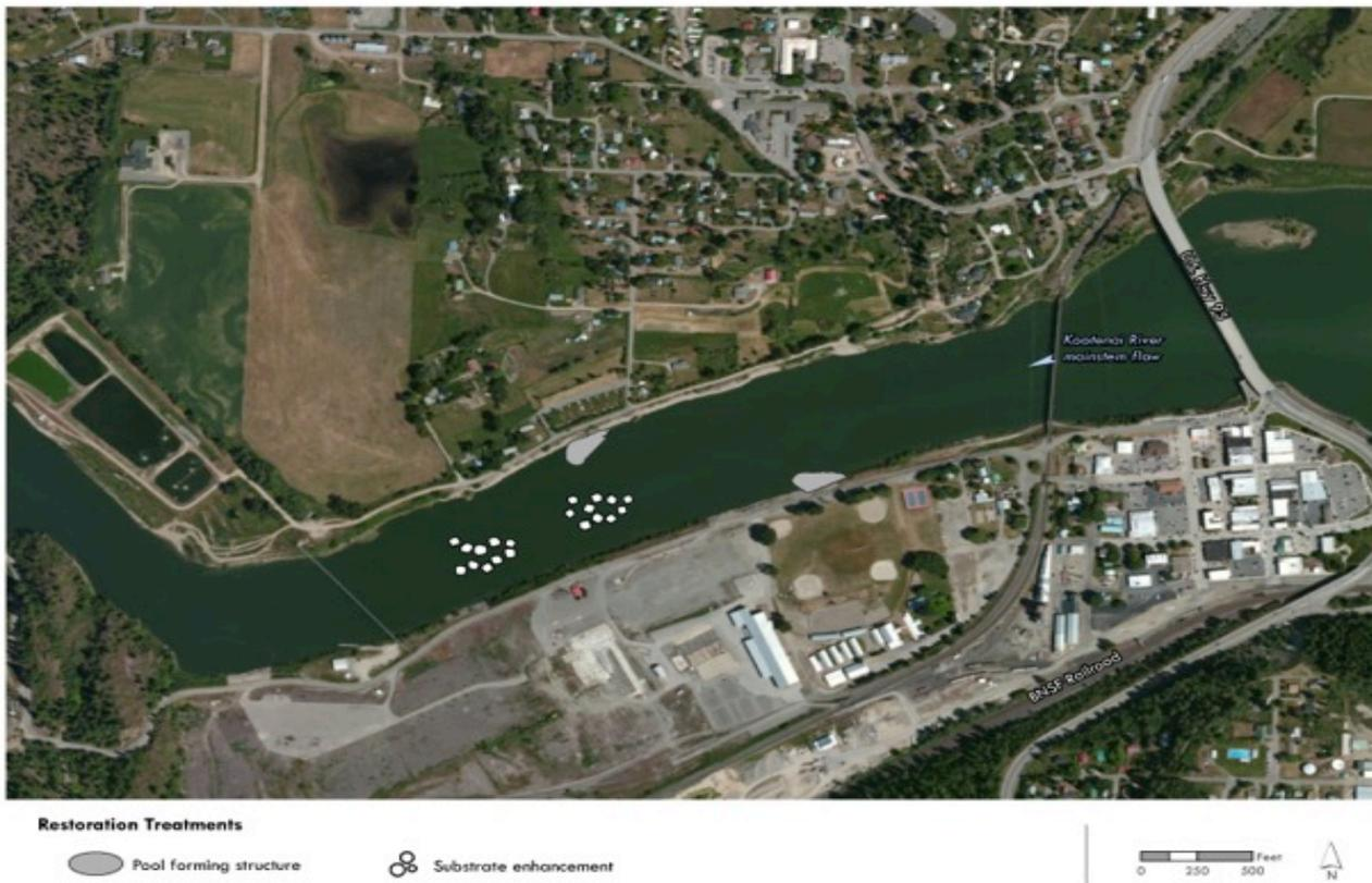
Figure 1. Straight Reach project illustration with pool-forming structures and substrate clusters.
